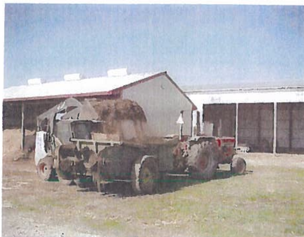
Figure 1. Composting rapidly decomposes swine mortalities, producing a soil-like product that can be spread on cropland. (Photo by Tom Glamville, Iowa State University.)
